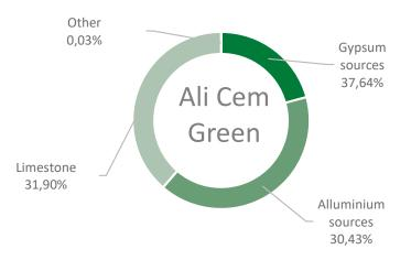
ALI CEM GREEN contain a high percentage of recycled materials used as aluminum sources. This particularity implies savings in natural resources and energy which would otherwise have been consumed. The aluminum based recycled materials result from the production of secondary aluminum and as such are classified as pre-consumer recycled materials according to the standard ISO 14021. Following rules set in this standard, the recycled material content of ALI CEM GREEN at 37.1%.
