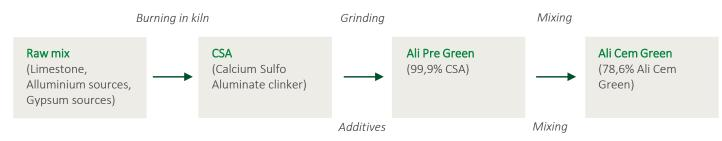
The overall composition of the products under study and the energy input involved are provided below. This shows relative percentages of materials and energy sources used in producing **ALI PRE GREEN** and **ALI CEM GREEN**, without considering loss in mass during combustion.
